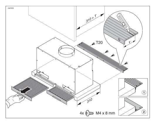
Pull the grease filters out of the slots in the front of the cooker hood housing.
